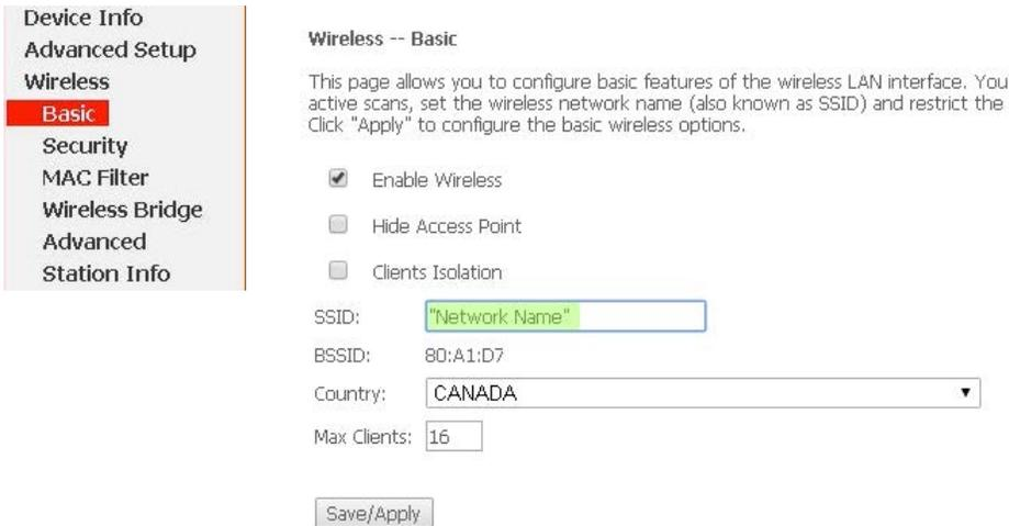
The screenshot shows a web interface for configuring wireless settings. On the left is a navigation menu with the following items: Device Info, Advanced Setup, Wireless, Basic (highlighted in red), Security, MAC Filter, Wireless Bridge, Advanced, and Station Info. The main content area is titled "Wireless -- Basic" and contains the following elements:
